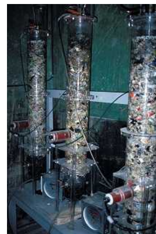
Photo 4. Column test setup(second stage)
