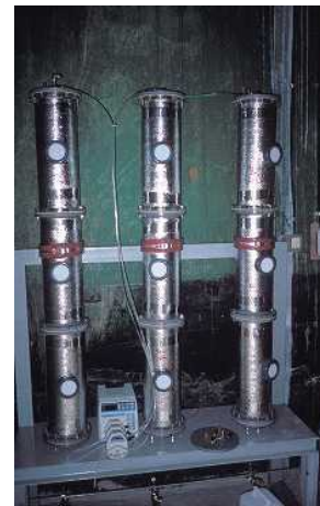
Photo 3. Column test setup
