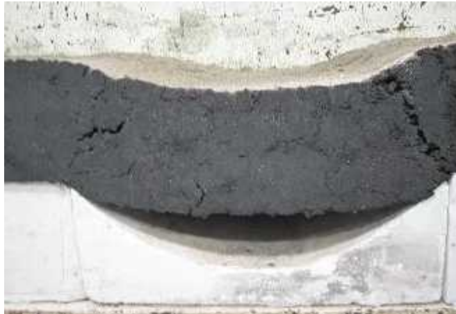
Figure 4 Appearance of cracks at the end of the fast deformation test (Case No.F1)
