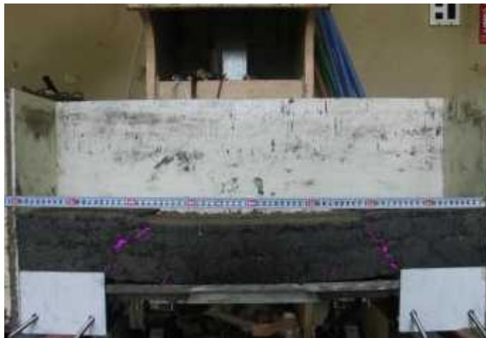
Figure 5 Appearance of cracks at the end of the slow deformation test (Case No.S3)
