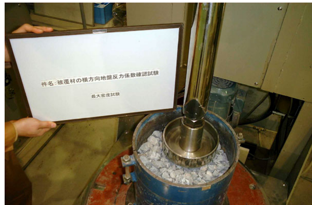
Figure 3. Maximum Density Test (Scoop Method)
