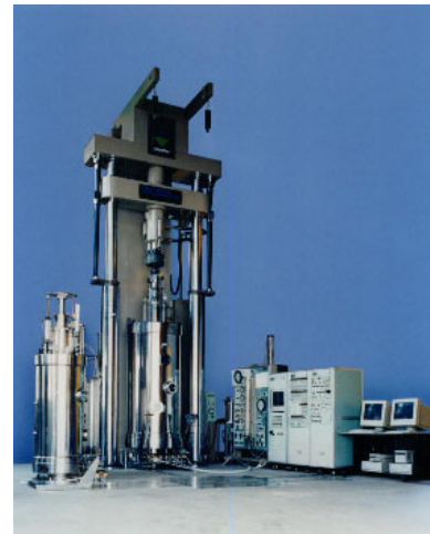
Figure 6. Large-Scale Tri-Axial Compression Test Device
