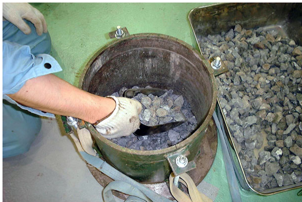
Figure 2. Minimum Density Test (Scoop Method)
