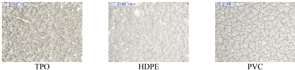
Figure 7. State of outdoor exposed surface (Okinawa)
