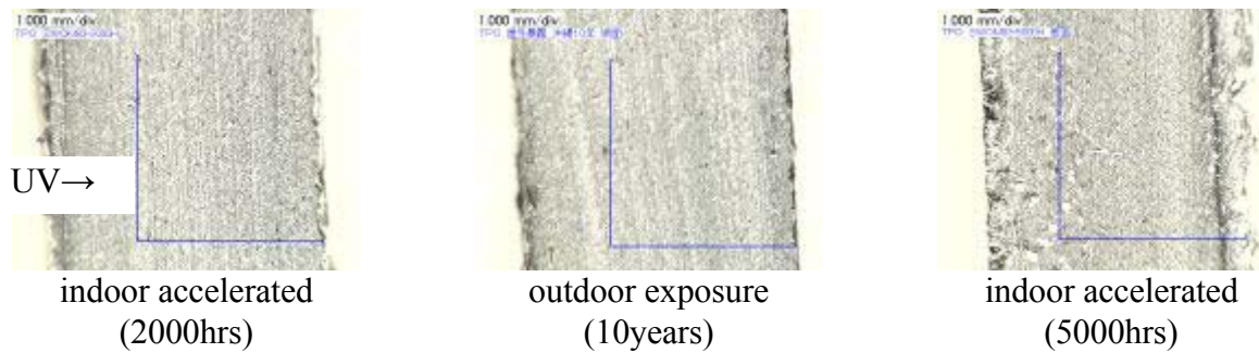
Figure 12. Cross section of TPO liner
